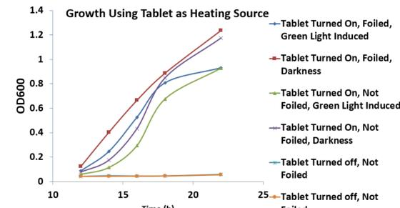
(Above) Heat generated by the tablet's processor while running the app can be used to incubate bacteria cultures. Growth was observed using the tablet as the sole heating element.
